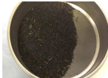
Fig. 2. Rice husk-derived biochar during sieving
