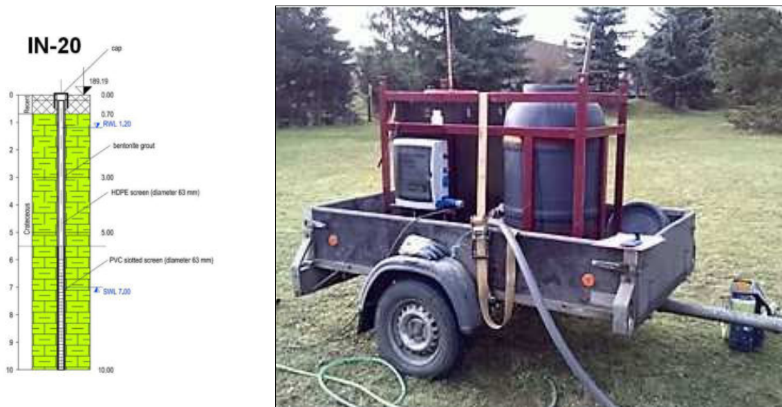
Fig. 3. Diagram of special application well (left) and TRAIN application device at the site (right).
